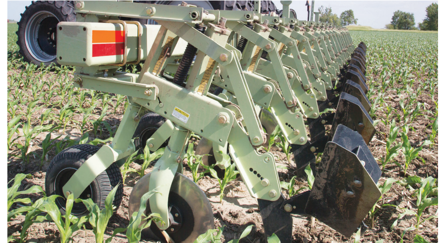
Single gauge wheel with western sweep and fertilizer tubes
