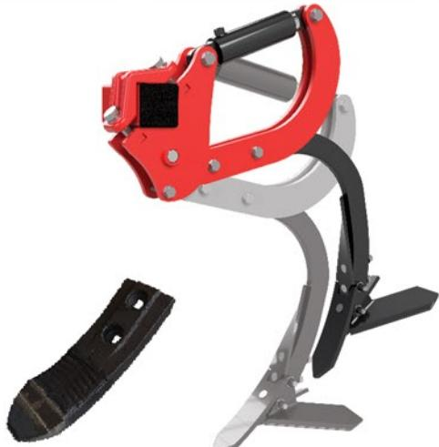
The tines are equipped with hydropneumatic protection and reinforced with tungsten carbide point as standard.
