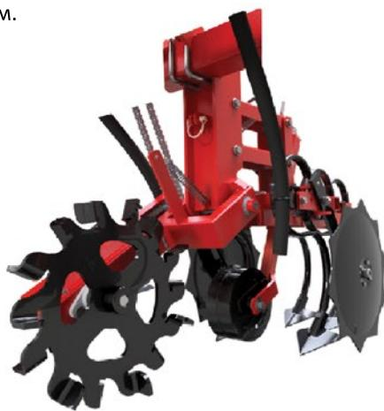
**EN** The tool gangs are attached to the main frame by parallel linkage assemblies that consistently keep each sweep moving independently at its desired depth in uneven terrain and independently of any fluctuations of the tractor. A gauge jockey wheel on each tool gang is responsible for accurate depth control.
