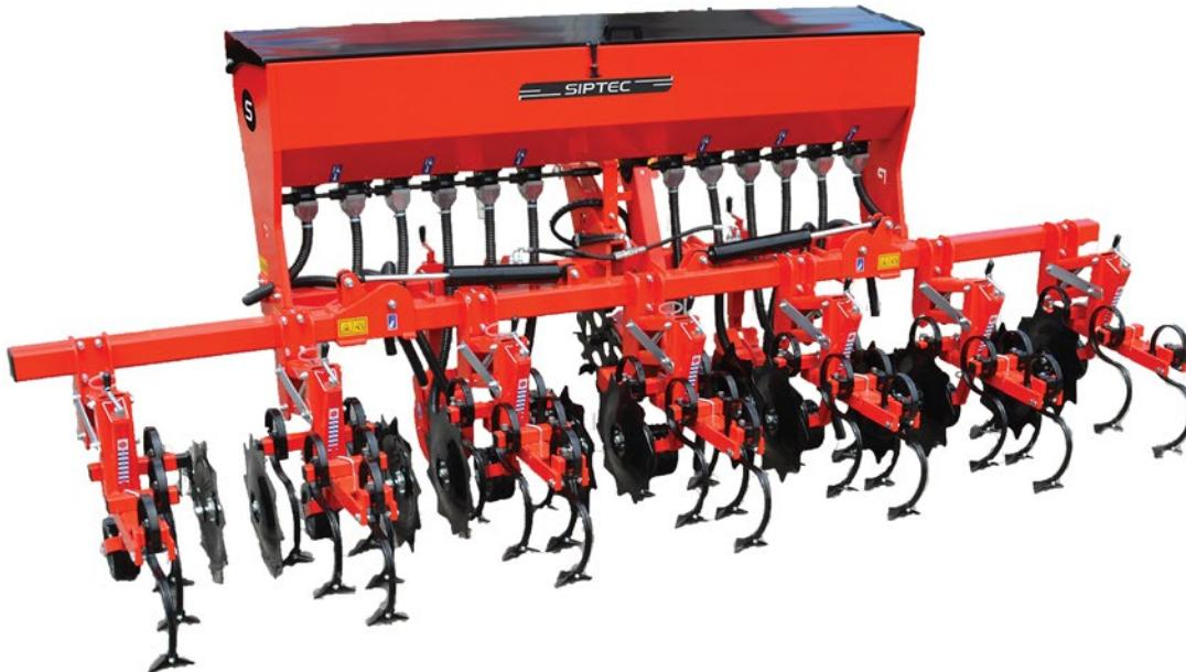
**EN** The painted steel fertilizer distributor is an optional feature while the hopper (stainless steel on demand) capacity ranges from 325 to 750 liters. The volumetric distribution is very accurate in both sides thanks to volumetric elements which are controlled by a sliding gear powered by a ground driven wheel.
